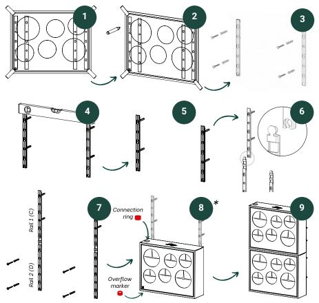
\*Always insert the connection ring into the pouring opening of the lower box and insert the overflow marker into the water tank.
